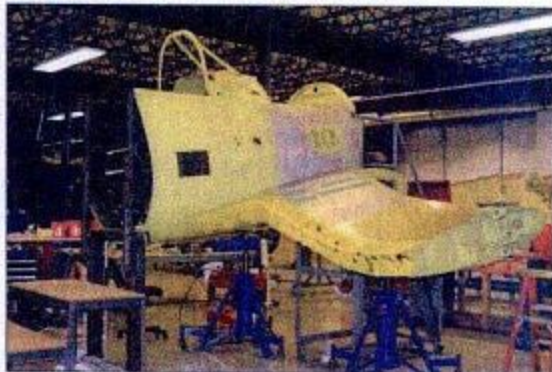
ABOVE The centre section of a Vought F4U-4 Corsair under restoration in Westpac's state-of-the-art restoration workshops at Colorado Springs.
